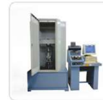
Computerized pullout testing machine
