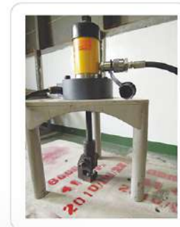
Pull out test
